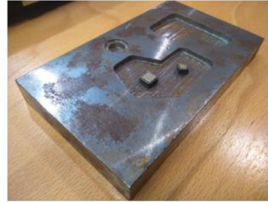
(c) Adding bosses by laser cladding
