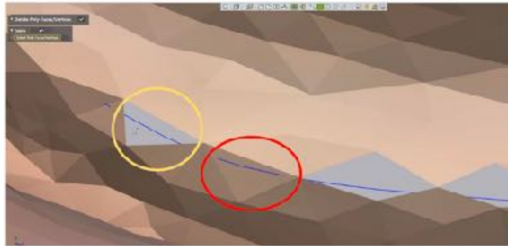
Fig. 37 Measurement of the total length of sharp and identifiable margins by evaluation of polygons forming the margin line in the 3D model. In the above example, the portion of the margins in red circle was left because it could be clearly distinguished by the edge of the polygon, while the portion of the margins in yellow circle was deleted because it appeared as a polygon face. The distinguishment between these two involved subjective judgements and was disputable.
